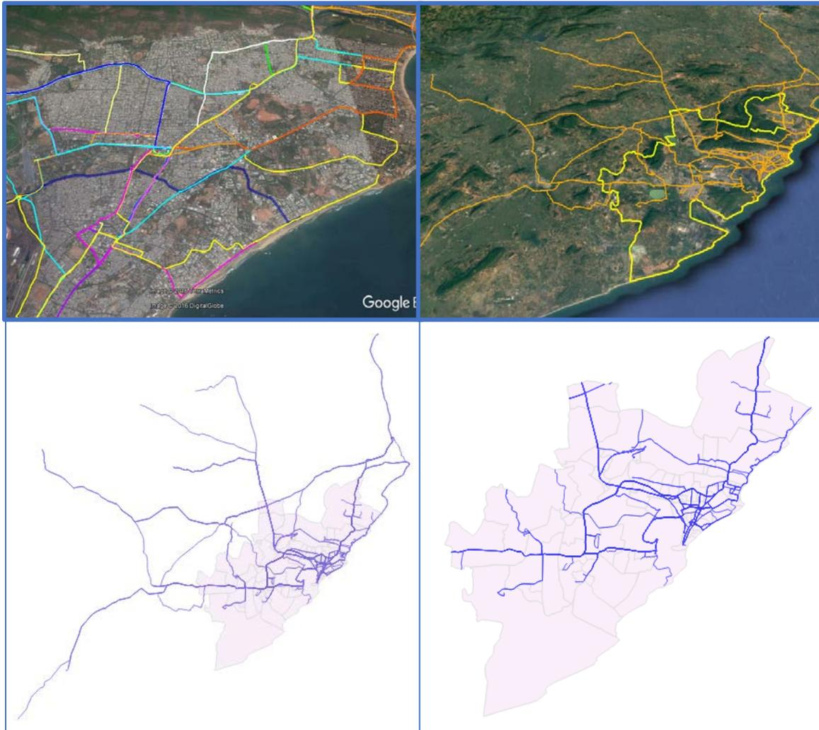
**Figure 12 Mapping the public transport routes and merging them with the road network**
